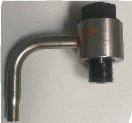
FIGURE 7: Actual photo of the nozzle.
