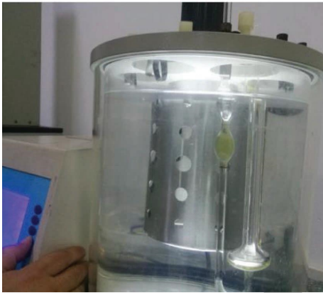
FIGURE 3: Viscosity test experiment.
