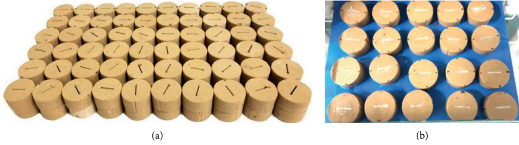
FIGURE 1: Fractured sandstone samples. (a) Sandstone specimens containing single fissure. (b) Sandstone specimens after freezing.
