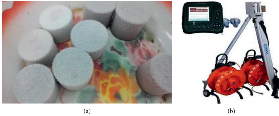
FIGURE 1: Photograph of the (a) frozen sandstone specimen and (b) equipment of the sonic wave test.
