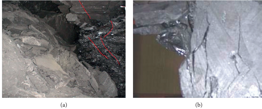
FIGURE 19: Coal fracture form under impact load. (a) Roadway; (b) coal body.
