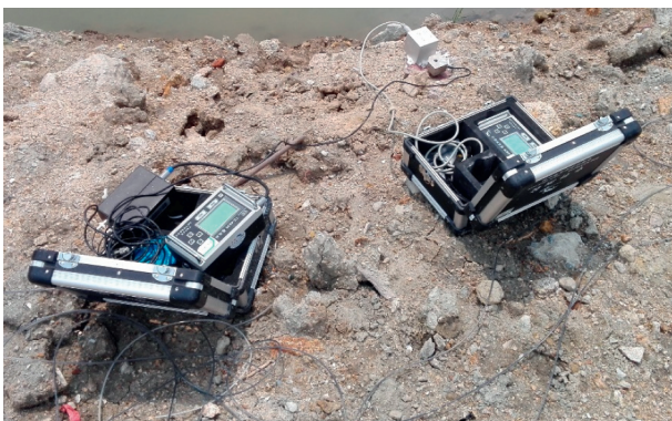
FIGURE 5: Arrangement of blasting vibration meters.
