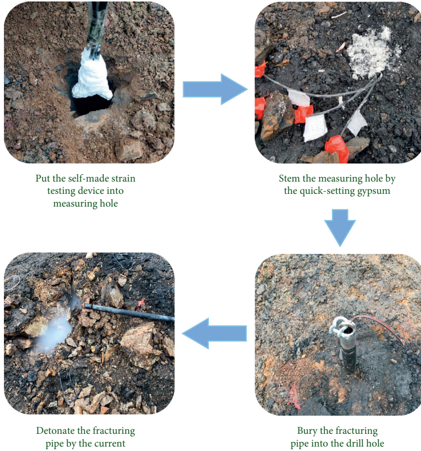
FIGURE 7: Installation process of the fracturing pipe and strain testing device.
