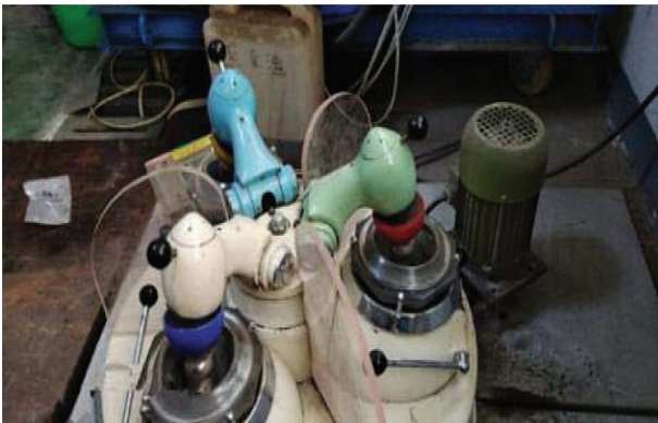
FIGURE 3: Carbonaceous rock sample grinding process from Hebailu.
