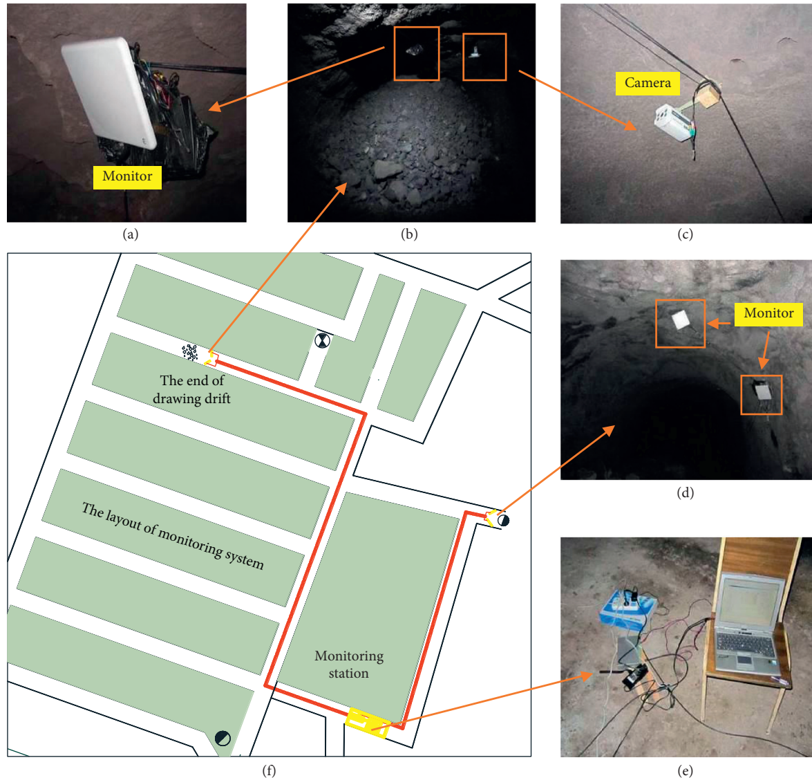
FIGURE 6: The layout of monitoring system: (a) monitors on the roof of the drift near drawing point; (b) monitors; (c) video on the roof of the drift near drawing point; (d) monitors next to the ore pass; (e) monitoring station.
