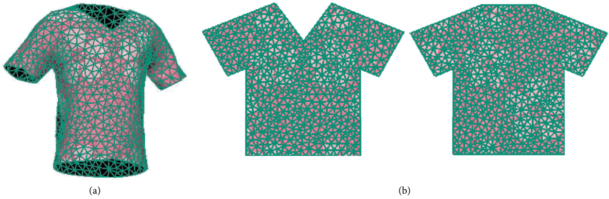
FIGURE 12: Energy-based flattening method for a coat: (a) original 3D mesh of a coat and (b) final 2D flattening of a coat.
