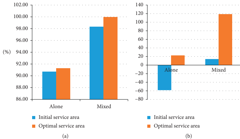
FIGURE 8: Comparisons of two operation modes before and after optimization. (a) Comparisons of average seat utilization. (b) Comparisons of number of vehicles required.
