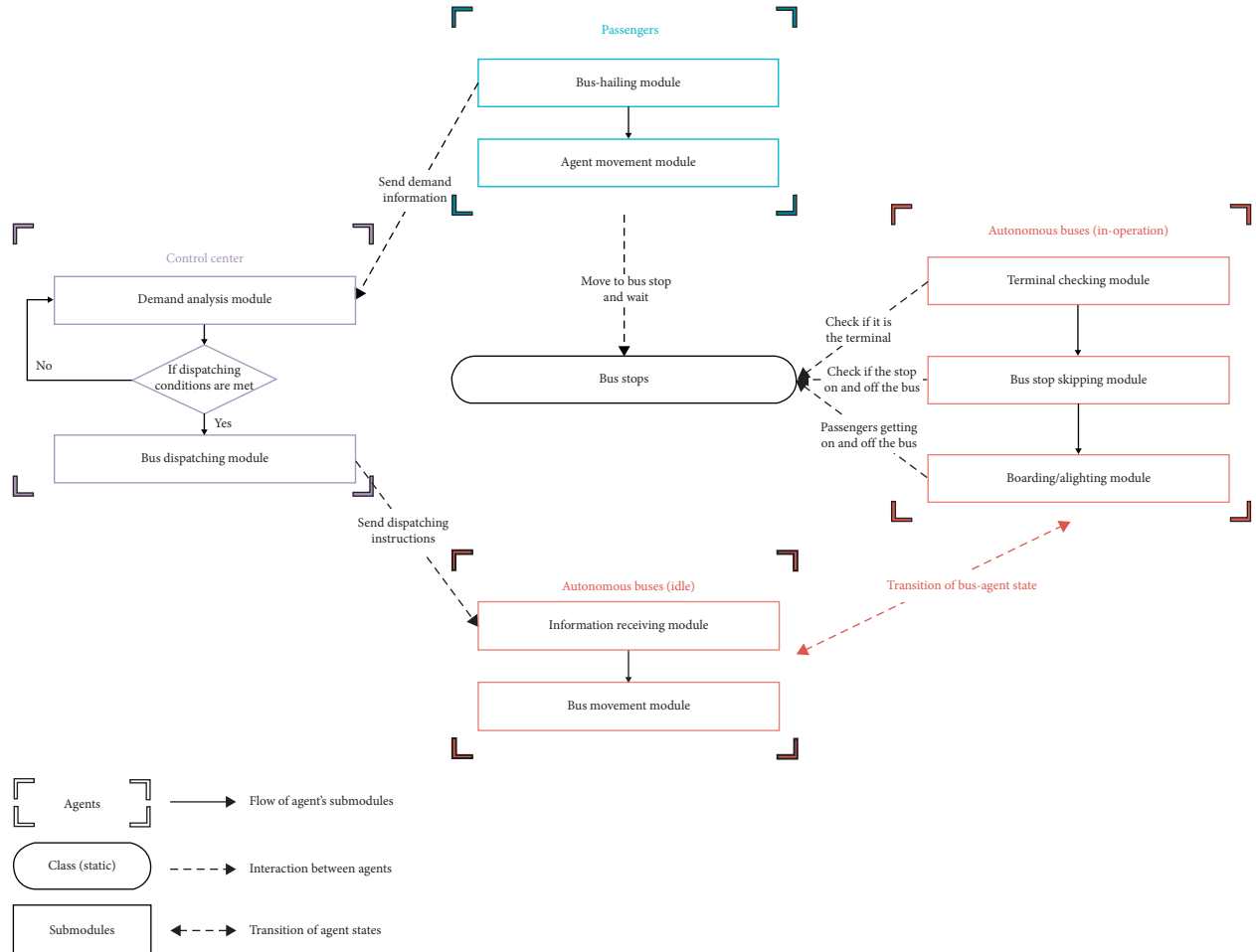
FIGURE 4: Agent-based simulation of passengers, control center, and autonomous buses.
