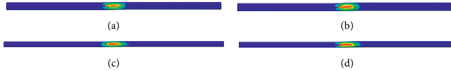
FIGURE 12: The cloud diagrams of plastic zone with different displacements under 90^\circ dip angle. Cloud diagram of plastic zone under strike-slip fault with (a) 0.9 m and (b) 1.1 m. Cloud diagram of plastic zone under thrust fault with (c) 0.9 m and (d) 1.1 m.
