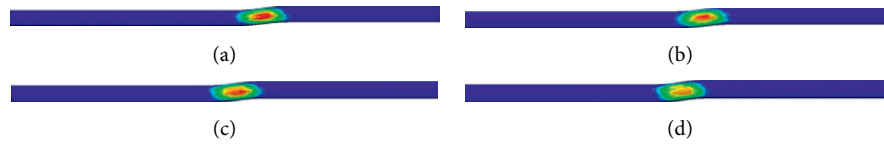
FIGURE 7: Plastic zone of lining under strike-slip fault with different dip angles. Cloud diagram of the plastic zone of the strike-slip fault with (a) 45° dip angle, (b) 60° dip angle, (c) 75° dip angle, and (d) 90° dip angle.
