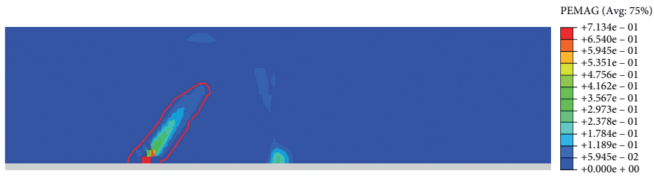
FIGURE 8: The cloud diagram of plastic zone of uniform round gravel soil model with a dislocation of 4.0 m.
