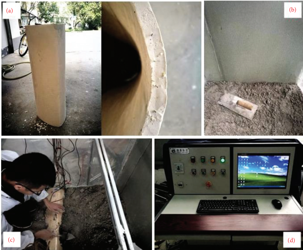
FIGURE 4: Model test setup. (a) Lining model. (b) Smoothing of lining. (c) Pouring surrounding rock. (d) Test operating platform.
