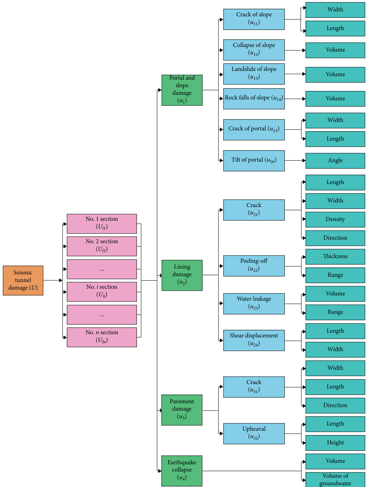
FIGURE 3: Structural diagram of AHP for the rapid assessment of the seismic damage level of tunnels.
