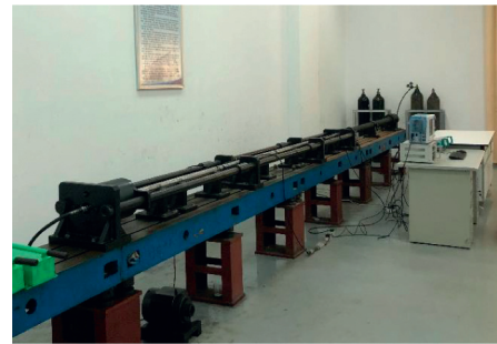
FIGURE 2: Split Hopkinson pressure bar test apparatus.
