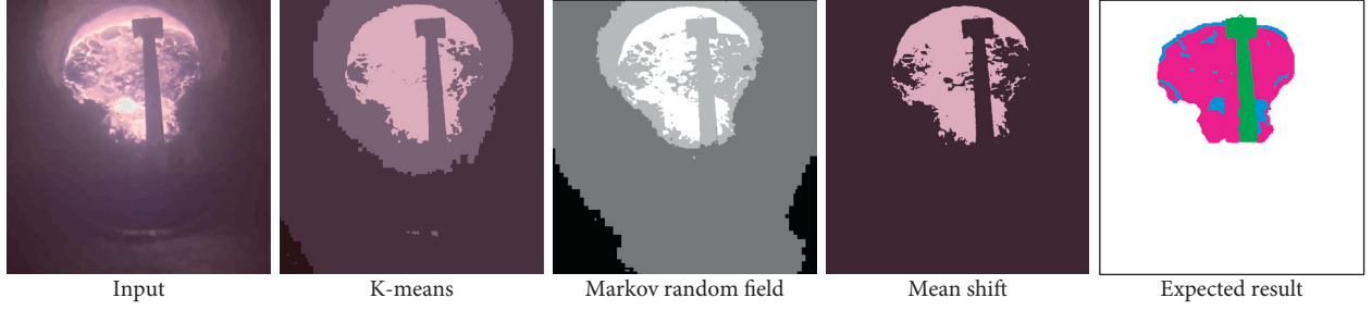
FIGURE 2: The segmentation results of traditional methods including K-means, Markov random field, and mean shift. The last column is the segmentation we expect. In the expected result, white, green, blue, and pink represent background, robotic arm, iron, and slag, respectively.
