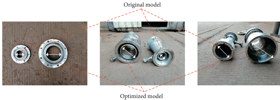
FIGURE 13: Comparison of annular ejector models. (a) Gland, (b) secondary inlet, and (c) outlet.
