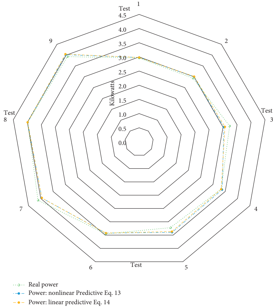
FIGURE 8: Drilling power real value compared against the results obtained with the nonlinear and linear predictive models.
