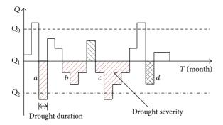
FIGURE 2: Diagram of drought identification using the theory of runs.
