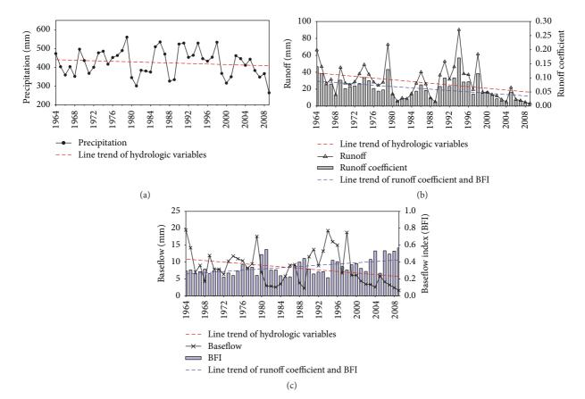
FIGURE 5: Variations of annual precipitation, runoff, runoff coefficient, baseflow, and baseflow index (BFI) over the Laohahe catchment since 1964. The red dashed line represents linear trend for hydrological variables (precipitation, runoff, and baseflow) and the blue dashed line for runoff coefficient and BFI.
