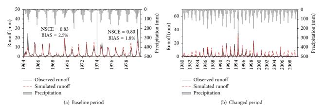
FIGURE 8: VIC simulated monthly runoff at the Xinglongpo hydrologic station for (a) the baseline period 1964–1979 and (b) changed period 1980–2009.
