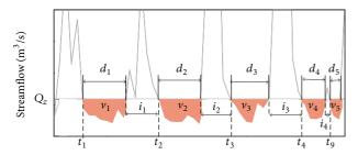
FIGURE 2: Illustration of threshold level method: time of occurrence,  $t_i$ , duration,  $d_i$ , deficit volume or severity,  $v_i$ , drought interval,  $i_k$ , and the threshold level,  $Q_i$ .
