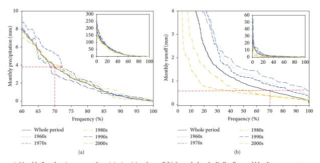
FIGURE 4: Monthly flow duration curves of precipitation (a) and runoff (b) for each decade. Dull yellow and blue lines represent curves for dry and wet decades, respectively.
