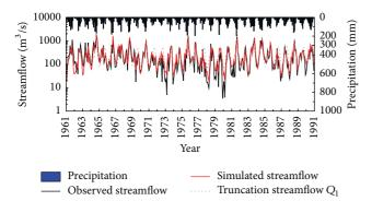
FIGURE 3: Observed and simulated monthly hydrographs at Huaxian station in the years 1961–1990.
