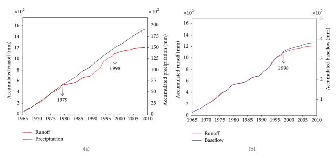
FIGURE 6: Double cumulative curves of (a) annual precipitation and runoff and (b) annual runoff and baseflow.
