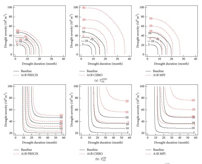
FIGURE 10: Bivariate joint return periods of drought duration and severity under baseline and A1B scenarios: (a)  $T_{\rm DS}^{\rm AND}$  defined by (7) and (b)  $T_{\rm DS}^{\rm OR}$  defined by (8).
