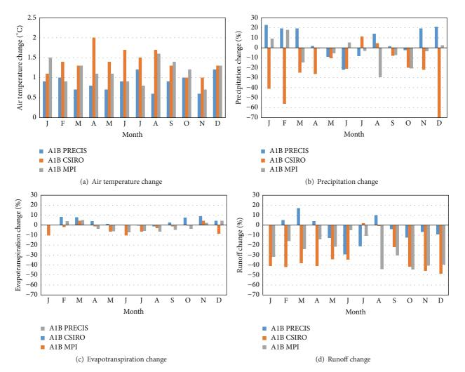
FIGURE 6: Projected changes in precipitation, air temperature, evapotranspiration, and runoff under A1B scenarios relative to baseline period.
