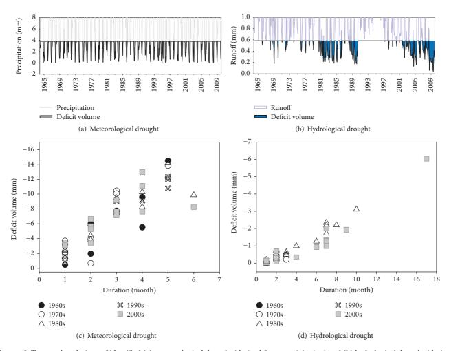
FIGURE 3: Temporal evolutions of identified (a) meteorological drought (derived from precipitation) and (b) hydrological drought (derived from runoff), and the scatterplots of drought duration and deficit volume for (c) meteorological and (d) hydrological droughts.
