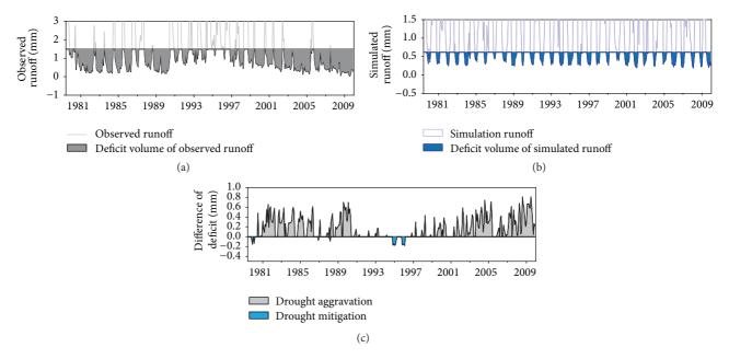
FIGURE 9: Identified hydrological droughts (with 70-percentile threshold derived from the baseline period) during 1980–2009 from (a) observed runoff and (b) simulated runoff series, and (c) is the difference between observed and simulated runoff series representing the net effect of human activities on drought.
