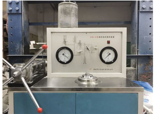
FIGURE 5: Vacuum saturation device (ZYB-1A).
