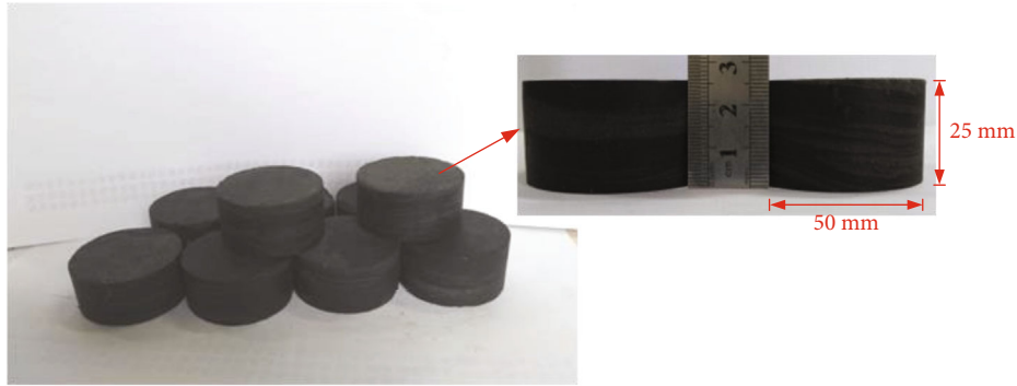
FIGURE 4: Mudstone specimen: diameter 50 mm and length 25 mm.
