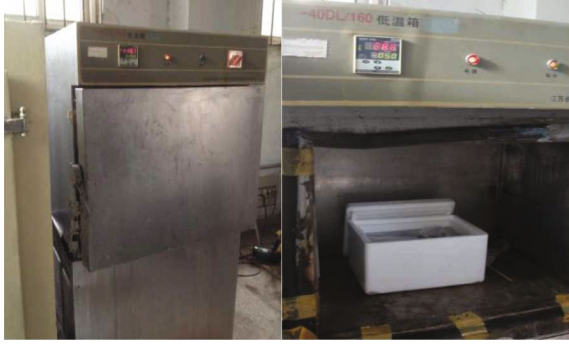
FIGURE 2: Freeze-thaw box.
