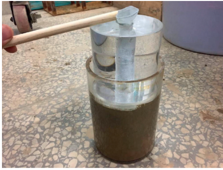
FIGURE 4: Set up of soil column with (drained) timber bolt before loading.
