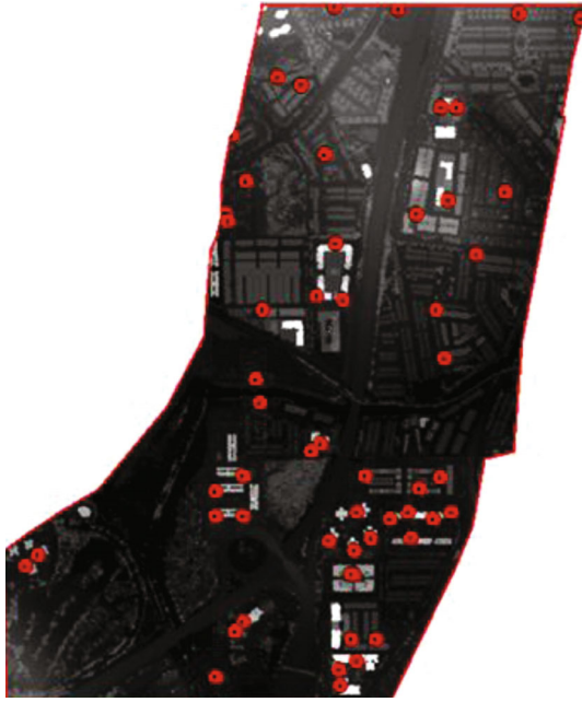
FIGURE 5: GCP distribution on DEM raster.
