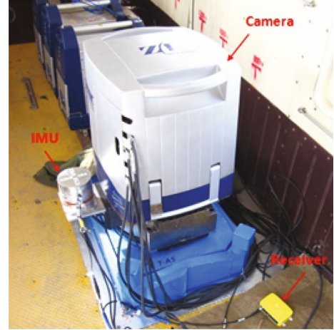
FIGURE 4: The assembly of sensors.
