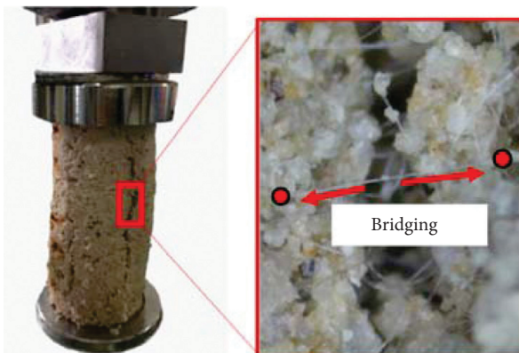
FIGURE 11: "Bridging" effect of fiber impedes the further development of crack [83].
