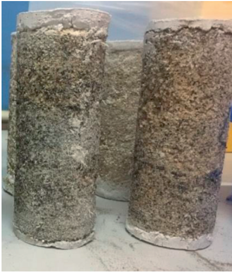
FIGURE 5: Sample of consolidated rubber sand.
