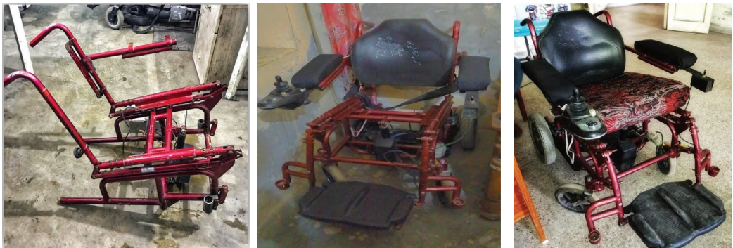
FIGURE 16: The final structure of wheelchair in sitting position.
