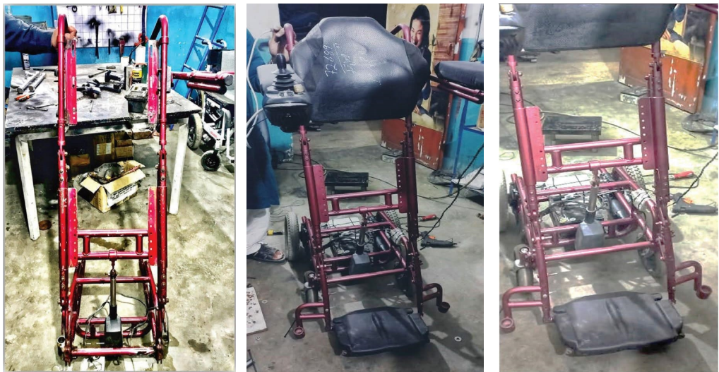
FIGURE 17: The structure of wheelchair in raised position.
