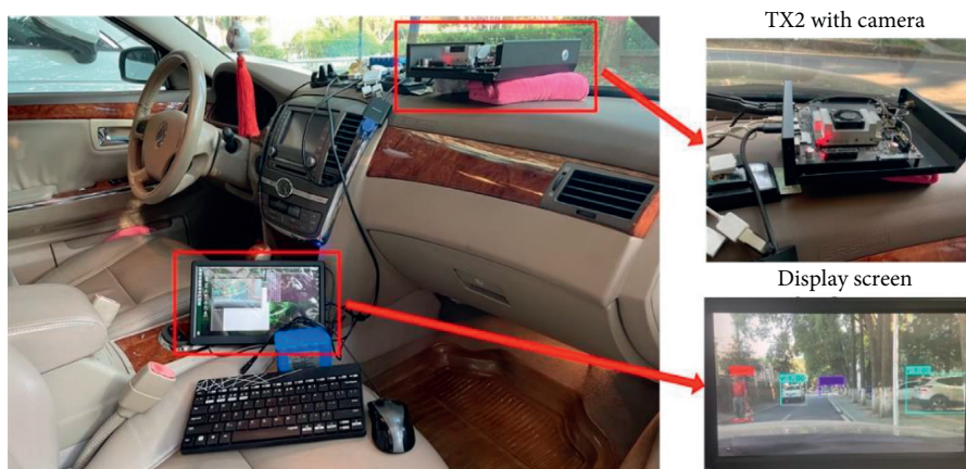
FIGURE 11: Vehicle application scenarios on NVIDIA TX2.
