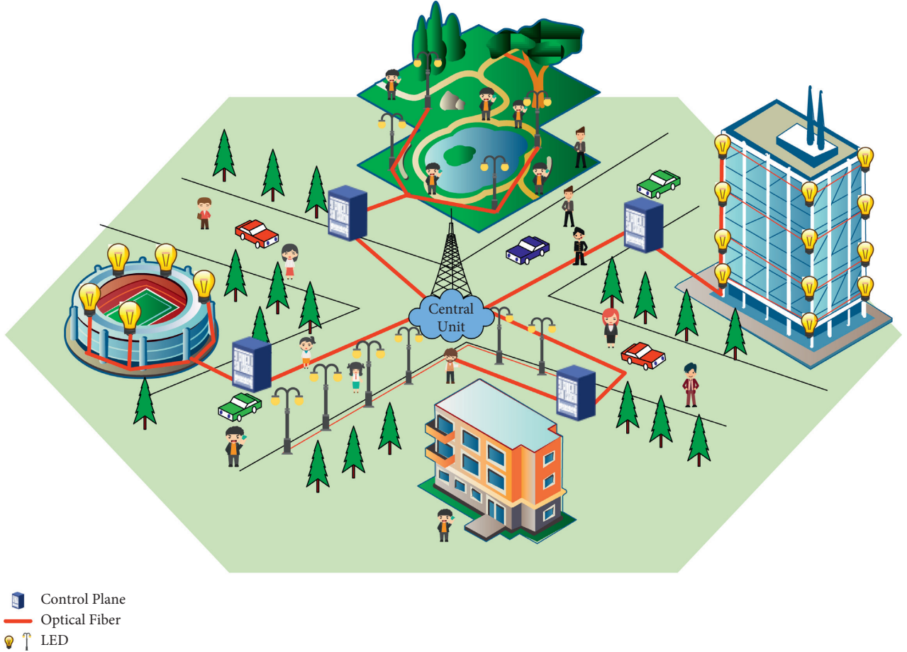
FIGURE 1: A new network framework based on SDN, UDN, and FVLC.
