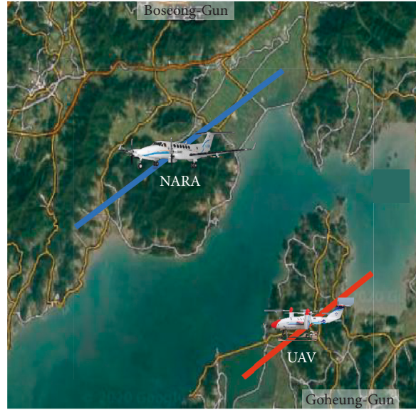
FIGURE 2: Target area and flight path of seeding by the UAV (red) and observation by the NARA (blue) over the southern part of the Korean peninsula on April 25, 2019.
