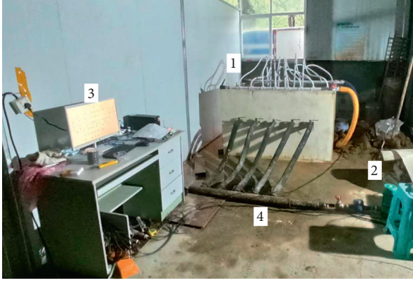
FIGURE 3: Scene photo of the model test system: 1, soil simulation system; 2, water pump; 3, measuring system; 4, water pipeline.
