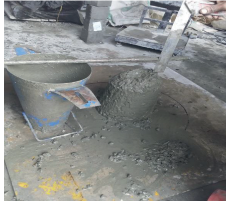
FIGURE 2: Slump test on the samples.
