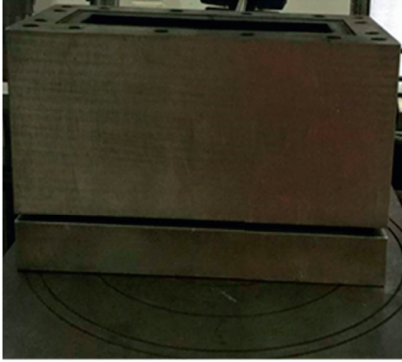
FIGURE 11: Linear flow guide chamber.
