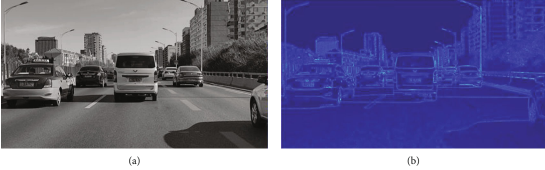
FIGURE 1: An example of the feature map in stereo matching. Left: grey image. Right: feature map.
