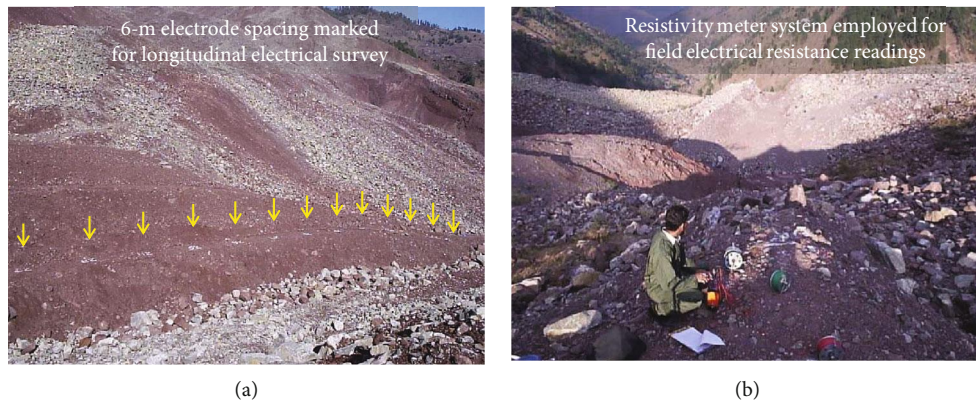
FIGURE 13: Field electrical resistivity survey in progress along the longitudinal survey line of the Karli spillway. The pictures illustrate (a) the marking of the electrode locations and (b) the resistivity system.
