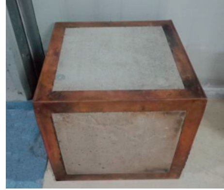
FIGURE 4: Edge angle seal of PPFRC.
