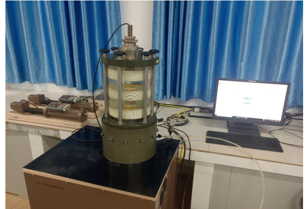
FIGURE 4: GDS cyclic triaxial testing system.
