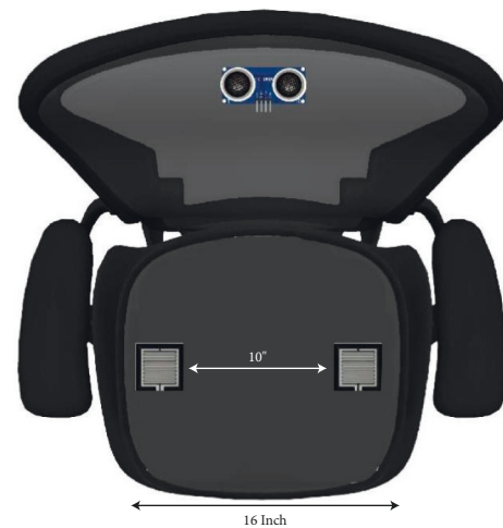
FIGURE 4: Arrangement 02: two FSR and one ultrasonic sensor.
