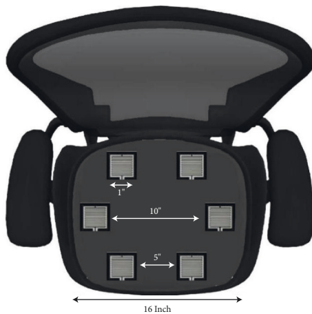
FIGURE 3: Arrangement 01, six sensors arrangement on a chair.
