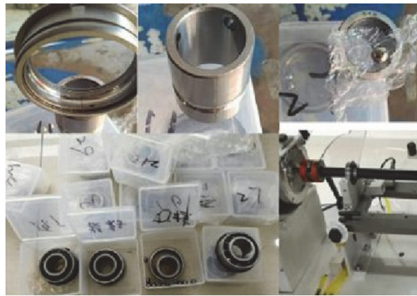
FIGURE 6: SER205 fault bearings.
