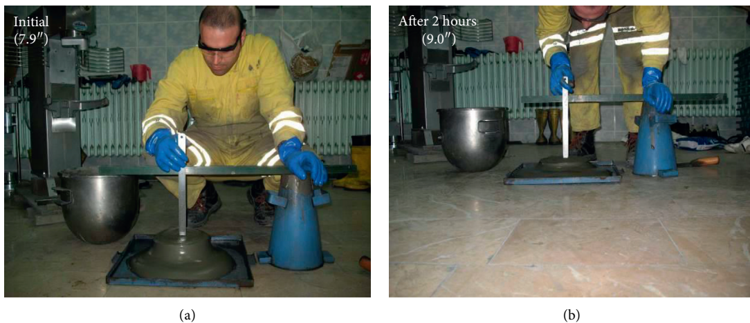
FIGURE 5: Slump levels of LSS-S/DT mixtures: (a) initial (7.9 inches) and (b) after 2 hours (9 inches).
