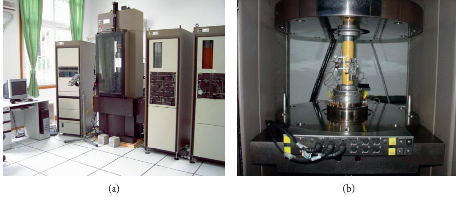
FIGURE 2: The test apparatus. (a) MTS815 rock mechanics test system. (b) Test specimen installation details.
