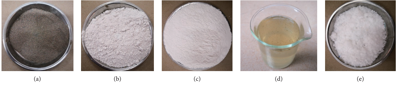
FIGURE 1: Main test materials. (a) Uranium tailings, (b) water-quenched slag powder, (c) quicklime powder, (d) liquid sodium silicate, and (e) sodium hydroxide.
