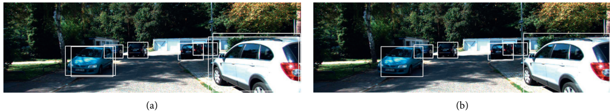
FIGURE 4: The comparison results by the detection method without NMS (a) and with NMS (b).
