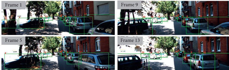
FIGURE 7: Result of the qualitative evaluation with the test sequence 0. Each vehicle is assigned a tracking ID as a reference.
