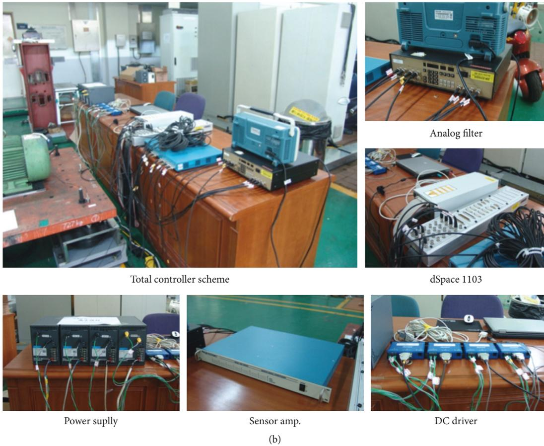
FIGURE 17: Experimental setup for 7-DOF system with electromagnetic hybrid mount. (a) Overall experimental setup for 7-DOF system. (b) Components for control.
