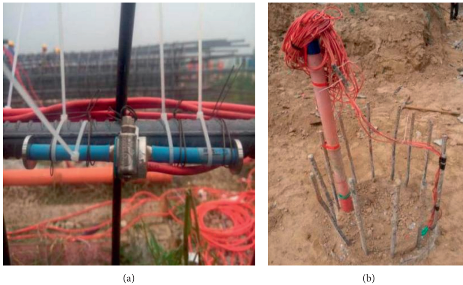
FIGURE 12: Binding and burial of strain gauges.
