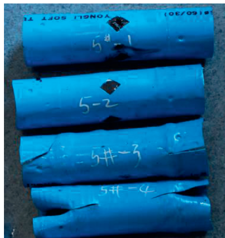
FIGURE 3: Coal samples after conducting the tests.
