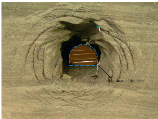
FIGURE 3: Zone disintegration of the model test.
