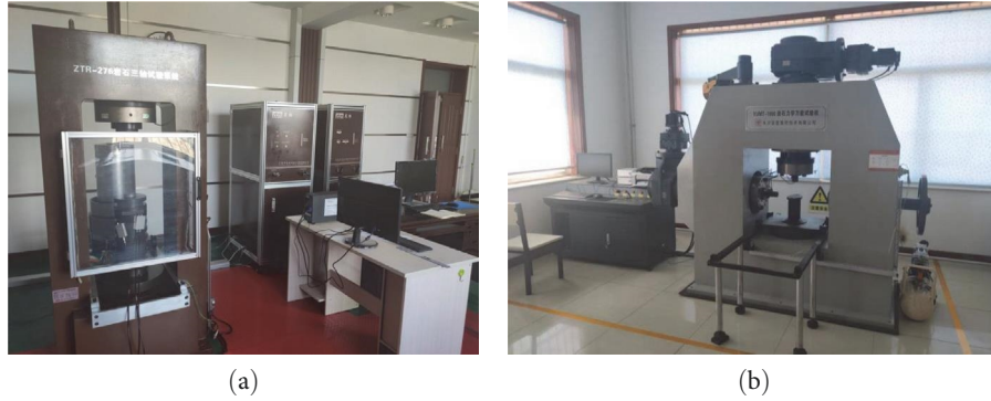
FIGURE 2: Laboratory rock mechanics test instrument: (a) ZTR-276 rock triaxial testing machine and (b) rock mechanics universal testing machine.
