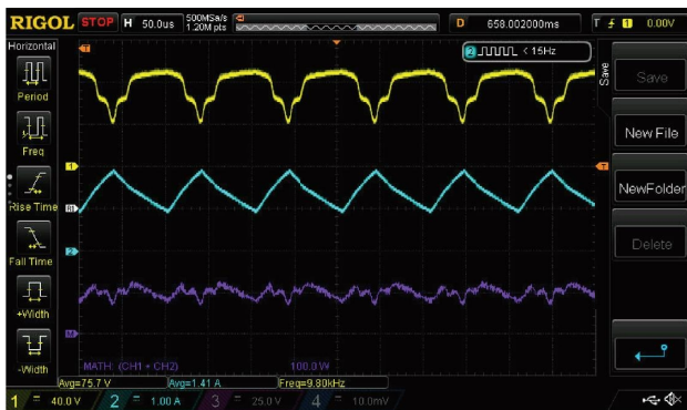
FIGURE 14: Experimental results for proposed GWO-ANFIS MPPT method for 4S configuration. (a) Pattern 1. (b) Pattern 2.
