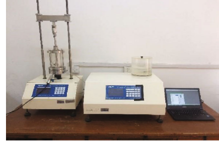
FIGURE 2: Fully automatic strain controlled triaxial apparatus.
