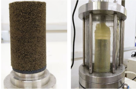
FIGURE 1: Samples before and during loading.
