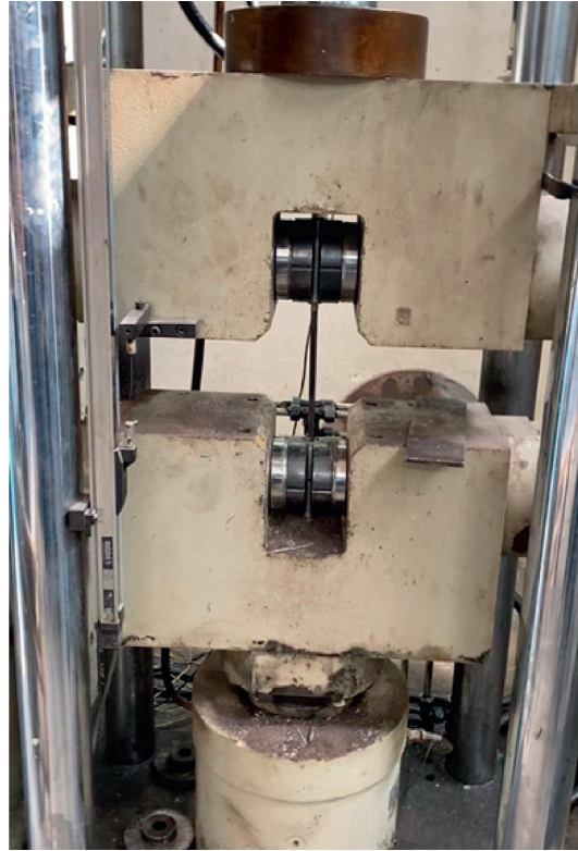
FIGURE 3: Tensile test of hybrid composite bars.
