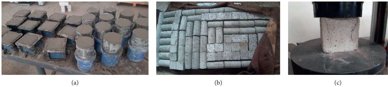
FIGURE 2: Preparation and testing of specimens. (a) Moulding of specimen. (b) Curing of specimen. (c) Compressive strength test setup.
