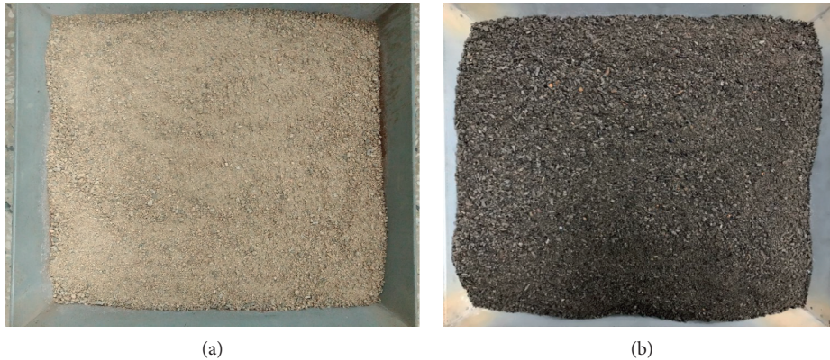
FIGURE 1: Natural fine aggregates and CBA aggregates. (a) Natural fine aggregates. (b) CBA aggregates.
