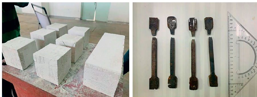
FIGURE 11: Test ALC blocks and steel coupons.
