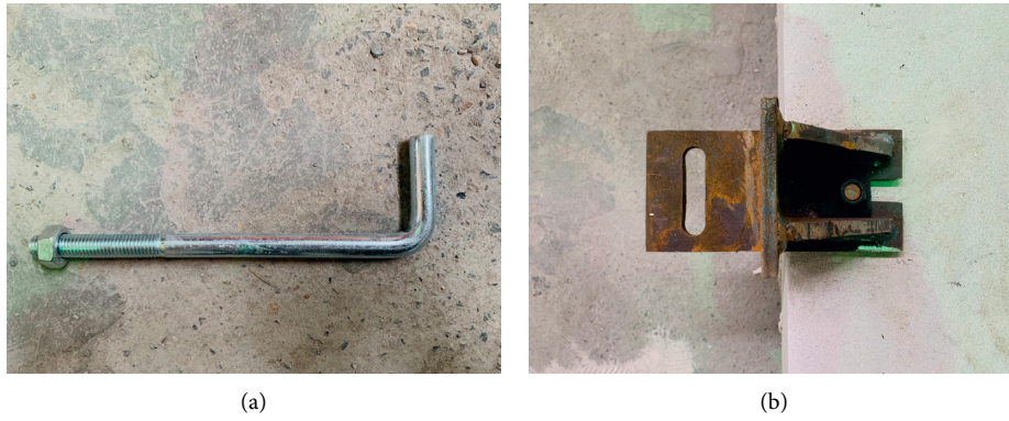
FIGURE 6: Test specimens. (a) L-hooked bolt (FW1). (b) Crossing ALC panel connector (FW2).
