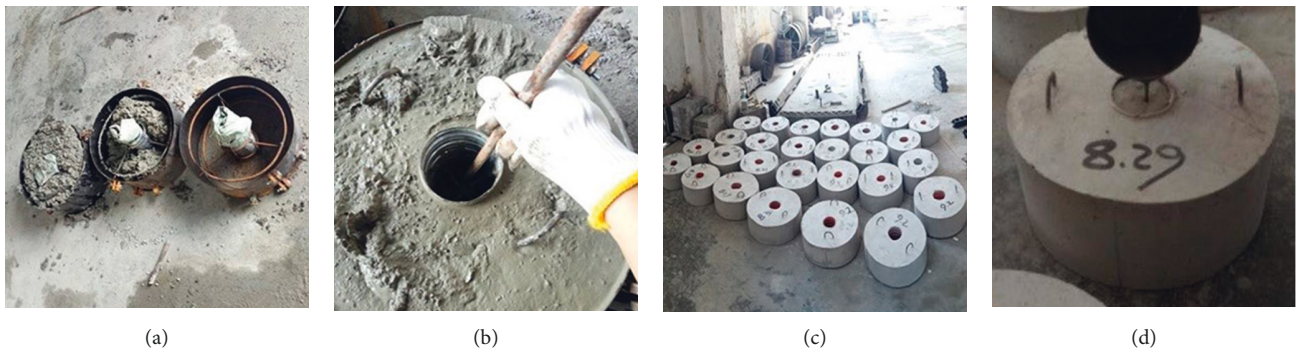
FIGURE 2: Specimen preparation, (a) Pour concrete, (b) Clean inside space, (c) Un-grouted specimen, (d) Grouted specimen.
