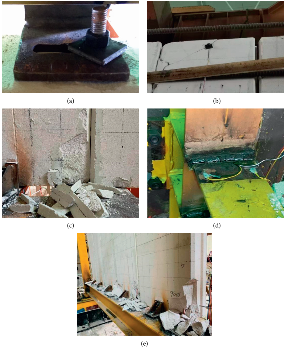
FIGURE 15: Test results of FW2. (a) Upper connector slipped within the bolt hole. (b) Cracks appeared at the upper bolt holes. (c) Corner of the panel back was broken off. (d) Weld of the beam-column node was chipped. (e) Corner and all mortar of joints were broken.
