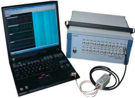
FIGURE 4: SAEU2S multichannel acoustic emission signal measurement system.
