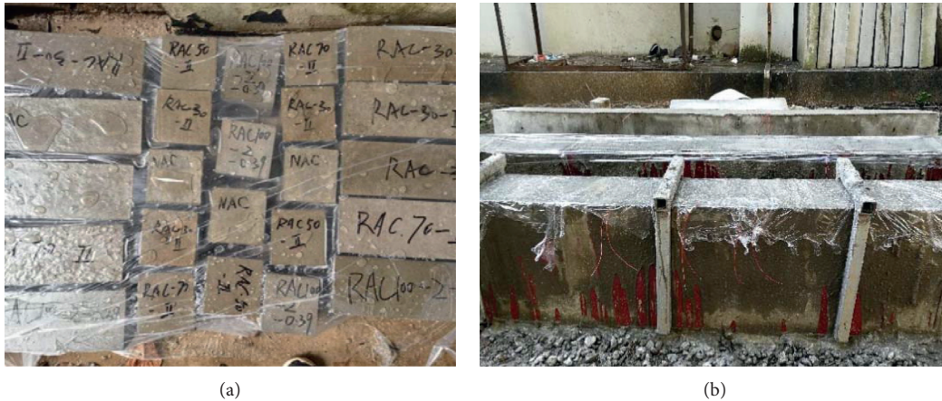
FIGURE 2: Experimental specimens. (a) Curing test block under the same condition. (b) Casting and forming.
