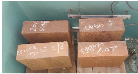
FIGURE 1: Curing of stabilized geopolymer mud blocks.
