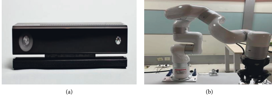
FIGURE 1: Interactive device diagram for intelligent massage positioning systems: (a) Kinect 2.0 devices; (b) xArm robotic arm devices.
