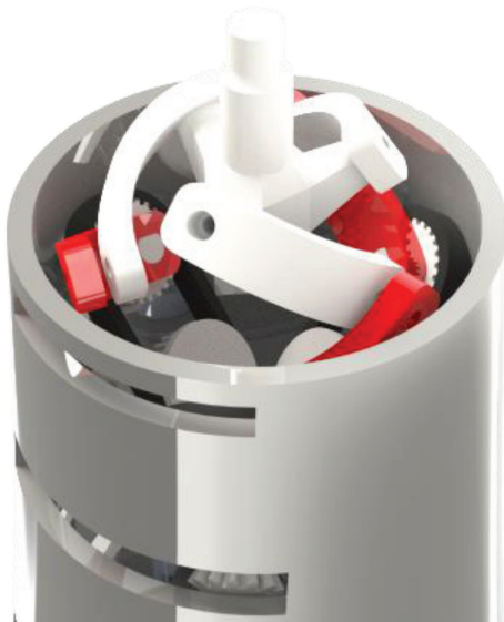
FIGURE 7: A CAD design of the parallel manipulator of the wrist.
