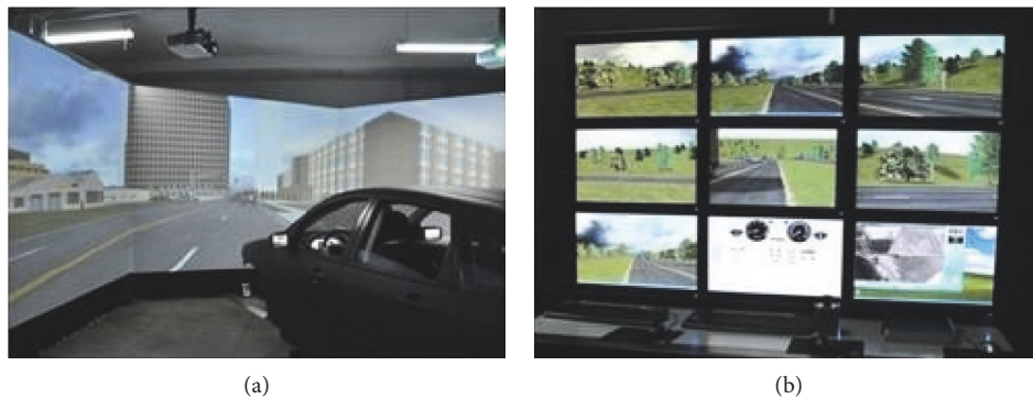
FIGURE 3: Illustration of BJTU driving simulator system. (a) Driving simulator; (b) monitoring and controlling systems.
