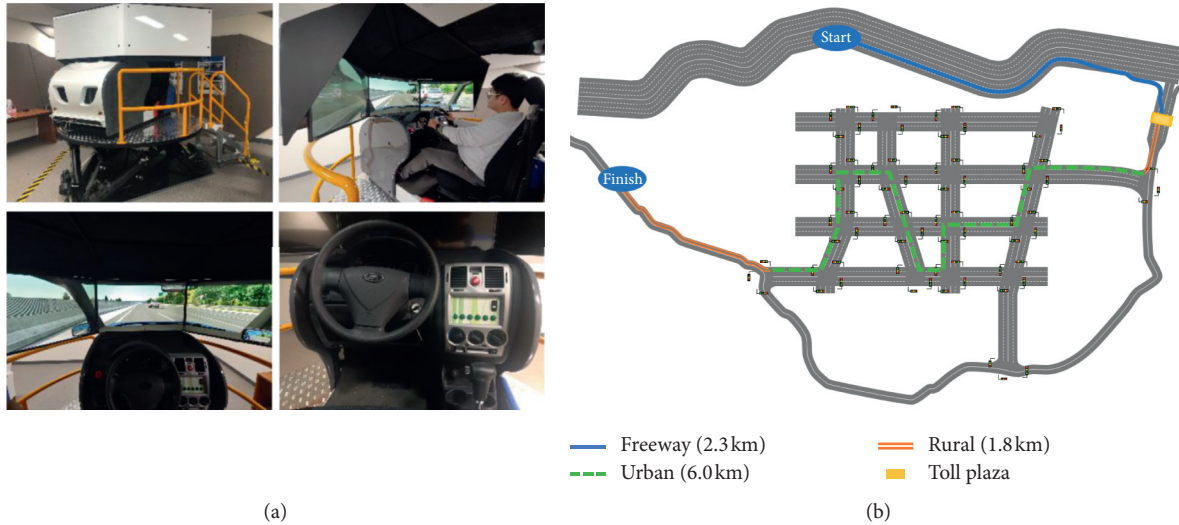
FIGURE 2: Driving simulator and scenario in this study: (a) the driving simulator set-up; (b) the designed route in the scenario.
