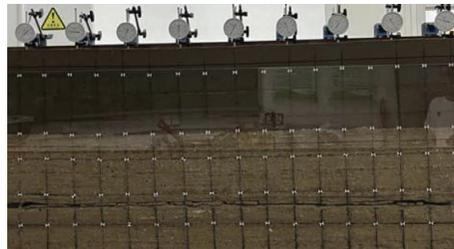
FIGURE 11: The roof caving with critical mining.
