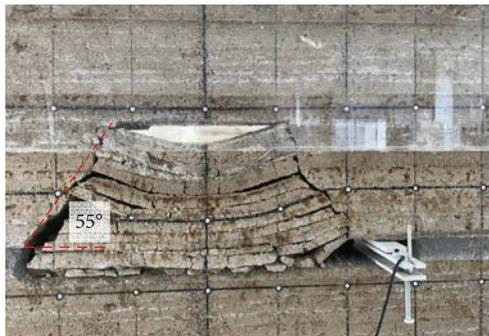
FIGURE 3: The first caving of main roof.
