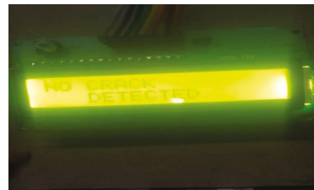
FIGURE 7: Displayed message on LCD, when no crack is detected.
