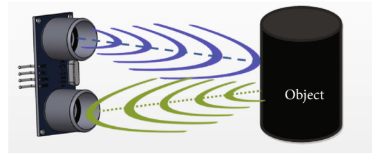
FIGURE 4: Ultrasonic wave travel in air.
