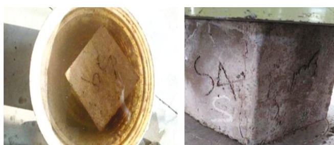
FIGURE 2: Concrete immersed 5% \text{Na}_2\text{SO}_4 and 5% \text{MgSO}_4 solution and surface change.
