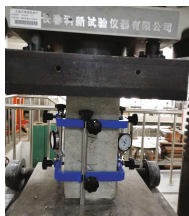
FIGURE 10: Elastic modulus test of substrate.
