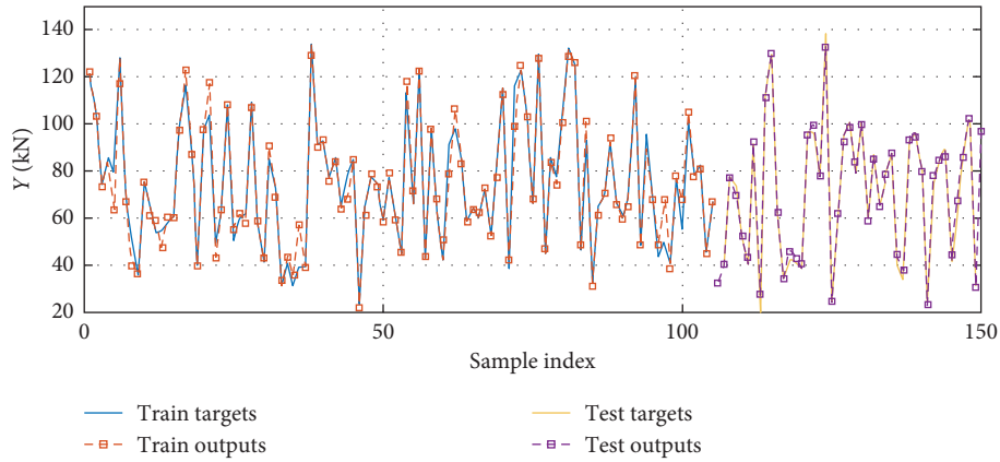
FIGURE 8: Experimental and predicted load-carrying capacity in function of sample index for the training and testing datasets.
