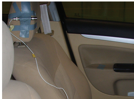
Figure 18: Microphone at driver's right ear position.
