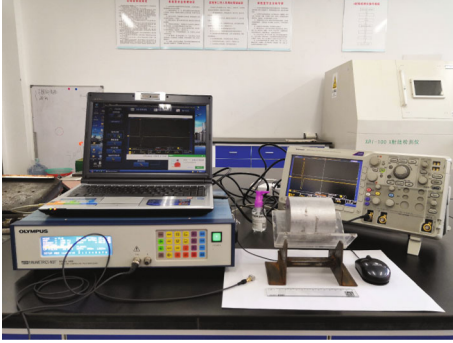
FIGURE 5: Ultrasonic testing equipment.
