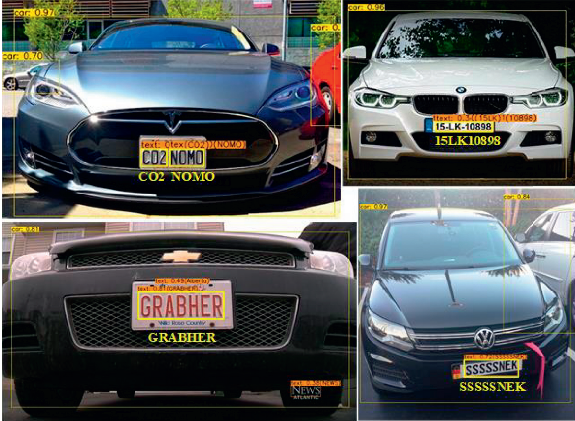
FIGURE 11: Examples of object-text detection and recognition results. There are some images of car with plate. We use yellow box to represent the detection results of car. The yellow solid boxes with overstriking are the text locations. The words in yellow are the word recognition results.
