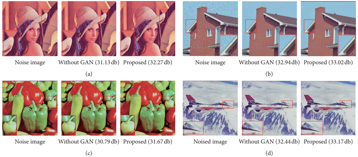
FIGURE 6: The compared experiments with and without GAN under the Gaussian noise of \sigma = 25 .
