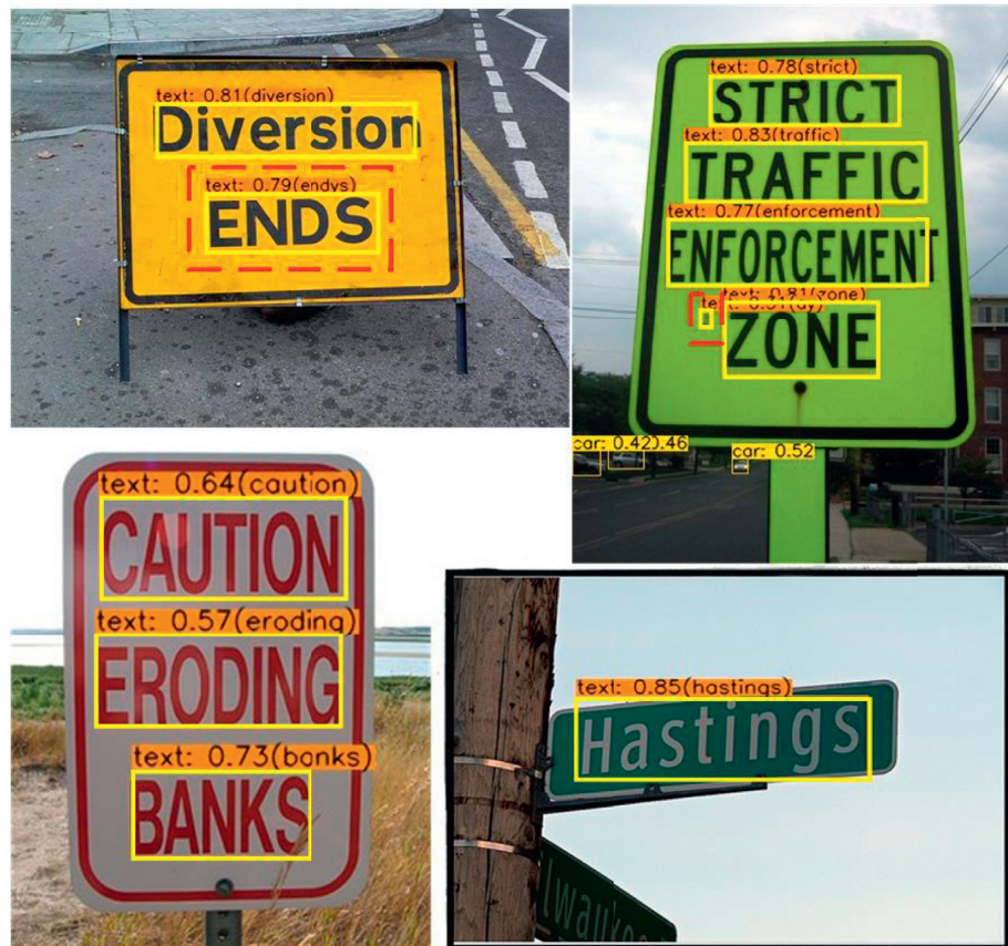
FIGURE 9: Examples of word spotting result. The yellow solid boxes with overstriking are the text locations. The words in parenthesis are the word recognition results. The red dashed boxes are the wrong word recognition.
