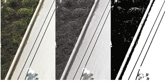
FIGURE 1: Applied correlation method on an image sample of power lines in the urban dataset.
