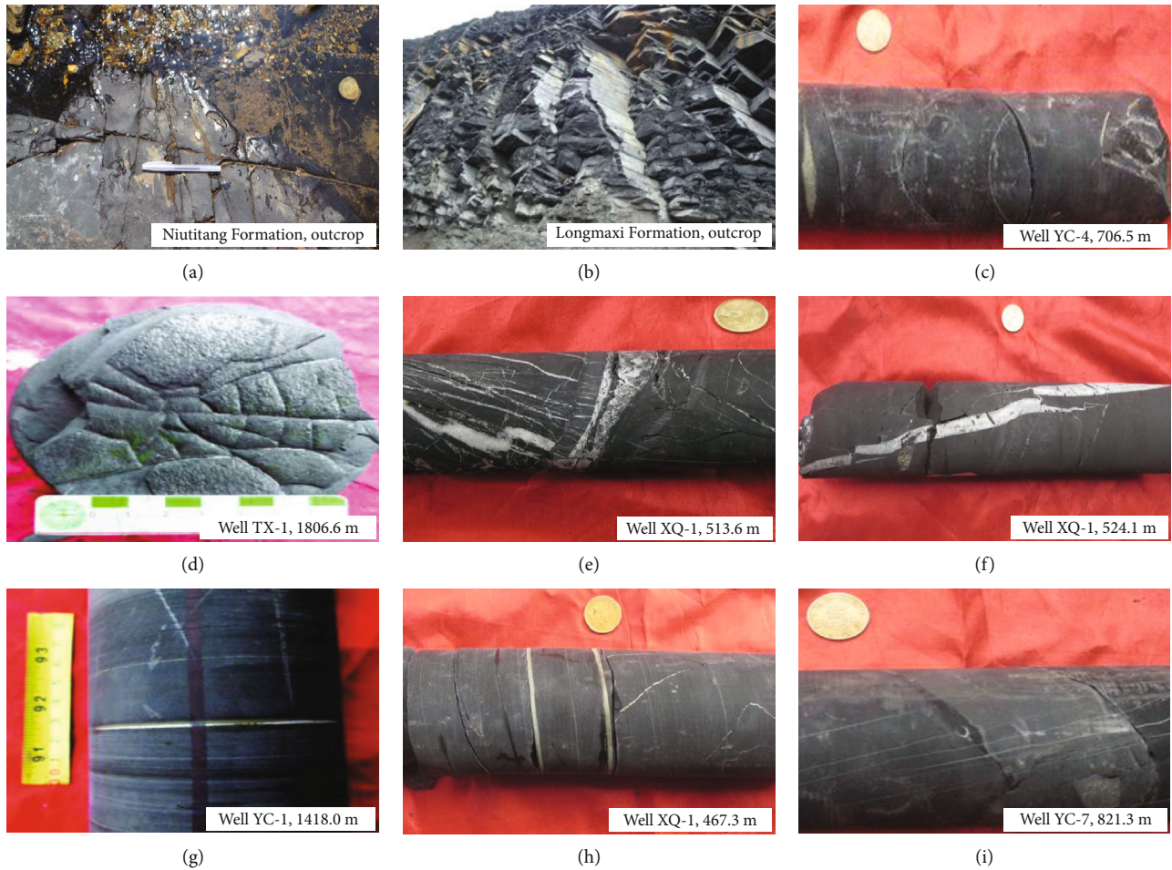
FIGURE 2: Shale fracture development characteristics in the target layer of southeastern Chongqing.
