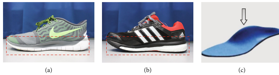
FIGURE 2: Profile of running shoes used in the experiment: (a) minimal shoe (MS), (b) heeled shoe (HS), and (c) sole profile of HS.
