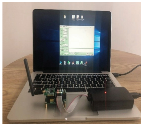
FIGURE 6: PC wireless transmission and reception node.
