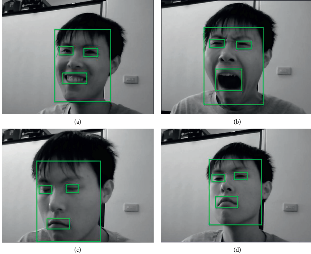
FIGURE 2: ROI positioning of eyes and mouth. (a) Normal state. (b) Yawning state. (c) Slow blink with nodding. (d) Sleepy state.
